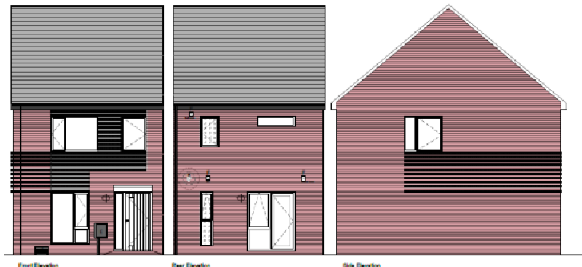
Elevations of one of the proposed house types (Type A)
